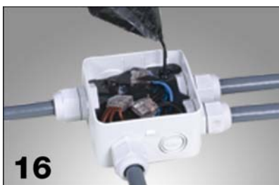
16 Pour the cast-resin slowly at one position to prevent inclosing of air bubbles.
