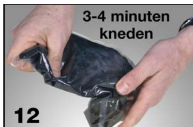
12 Knead the cast-resin into a homogeneous mass during 3-4 minutes. The mixture will become a little bit hot (35-40°C) due to the chemical process. Repeat step 11 every minute.
