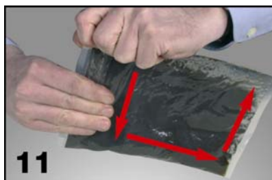
11 Press also on the edges of the bag in order to mix both components completely.
