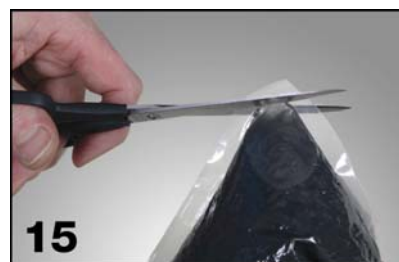
15 Cut a small hole in the mixing bag in order to form a spout.
