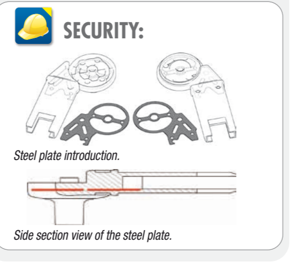
Automatic alum die-casting hinge with an inner steel plate strengthening.
